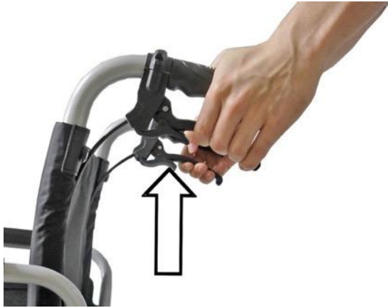
Fig.22: Operating the brake
