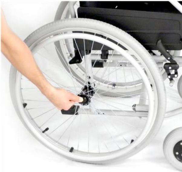
Fig. 7: Disassembling the rear wheel
