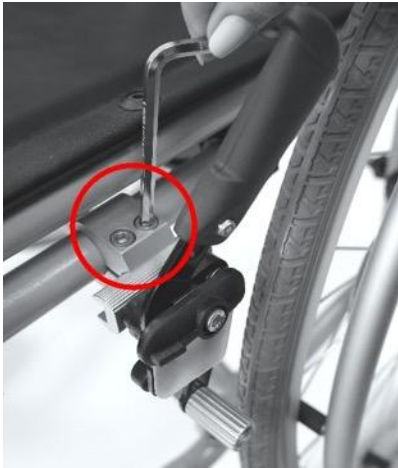
Fig. 10: Adjusting the brakes
