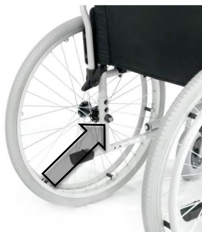
Fig. 8: Adjusting the height of the rear wheel
