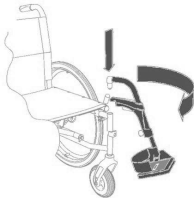
Fig. 5: Inserting the leg supports
