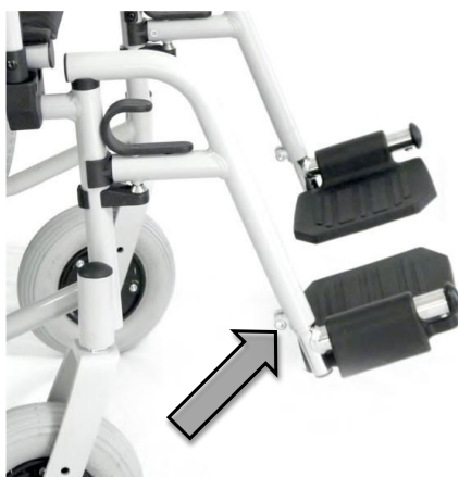
Fig. 6: Adjusting the lower leg length
