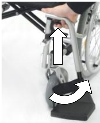
Fig. 14: Disassembling the footrests
