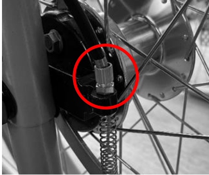
Fig. 13: Drum brake adjusting screw
