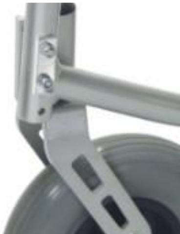
Fig. 9: Adjusting the height of the front wheel
