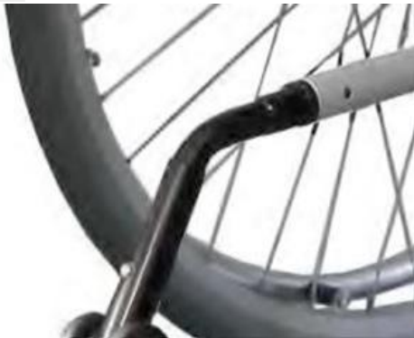
Fig. 19: Fitting the anti-tip supports
