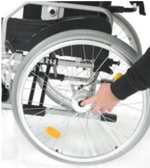
Fig. 7: Disassembling the rear wheel
