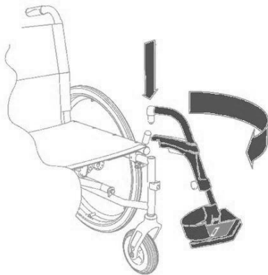
Fig. 5: Inserting the leg supports
