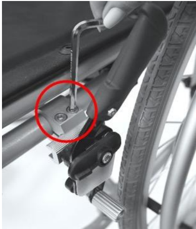
Fig. 10: Adjusting the brakes
