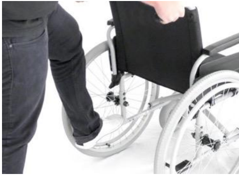
Fig. 18: Use of the tilting aid
