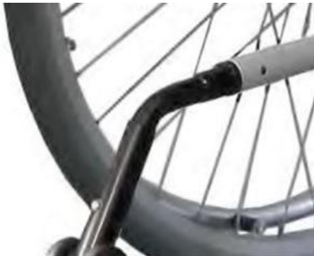
Fig. 19: Fitting the anti-tip supports
