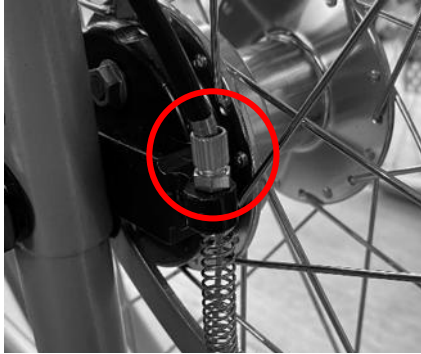
Fig. 13: Drum brake adjusting screw
