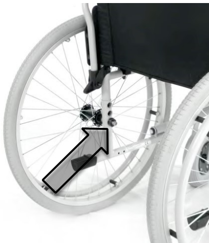
Fig. 8: Adjusting the height of the rear wheel
