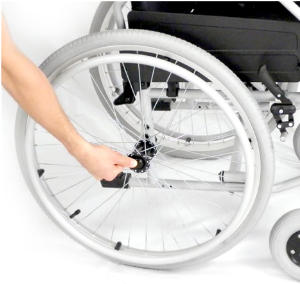
Fig. 7: Disassembling the rear wheel
