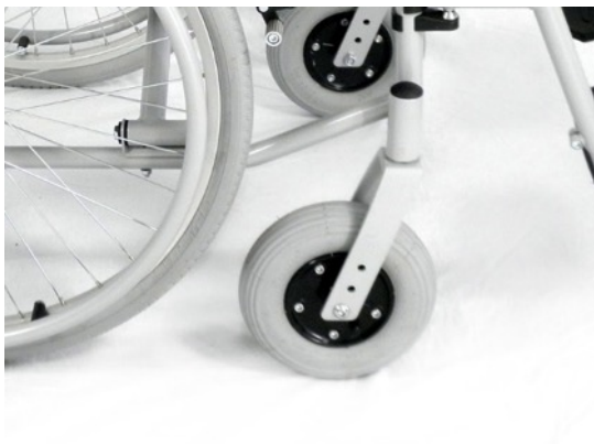
Fig. 9: Adjusting the height of the front wheel
