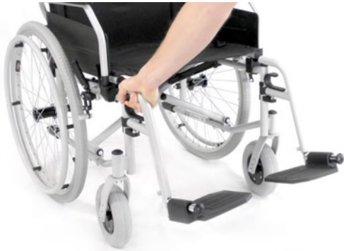
Fig. 14: Disassembling the footrests
