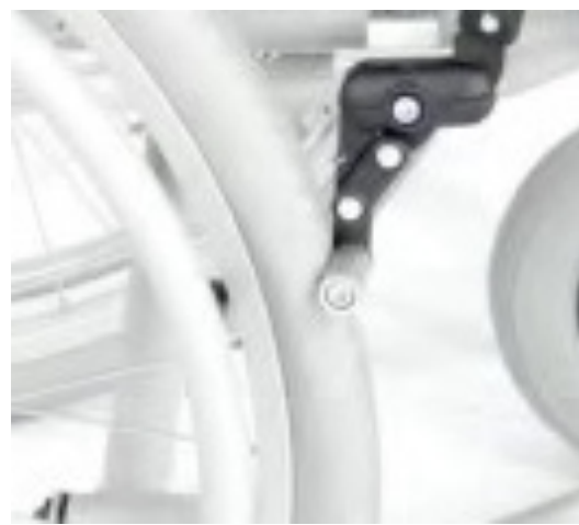
Fig. 12: Parking brake applied
