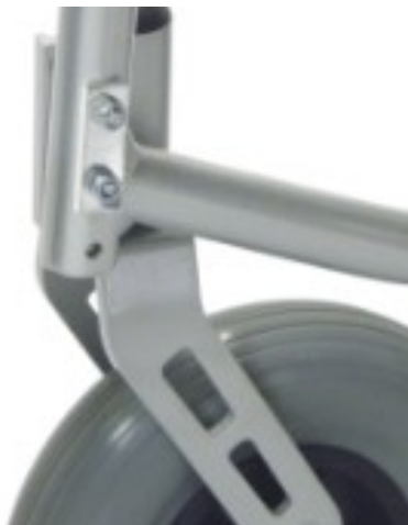
Fig. 9: Adjusting the height of the front wheel
