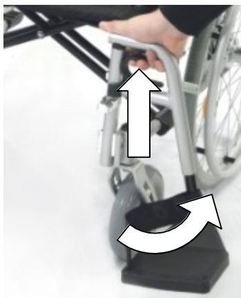
Fig. 14: Disassembling the footrests
