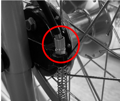
Fig. 13: Drum brake adjusting screw
