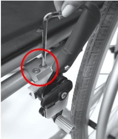
Fig. 10: Adjusting the brakes
