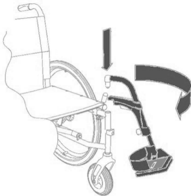
Fig. 5: Inserting the leg supports
