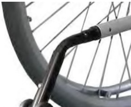
Fig. 19: Fitting the anti-tip supports
