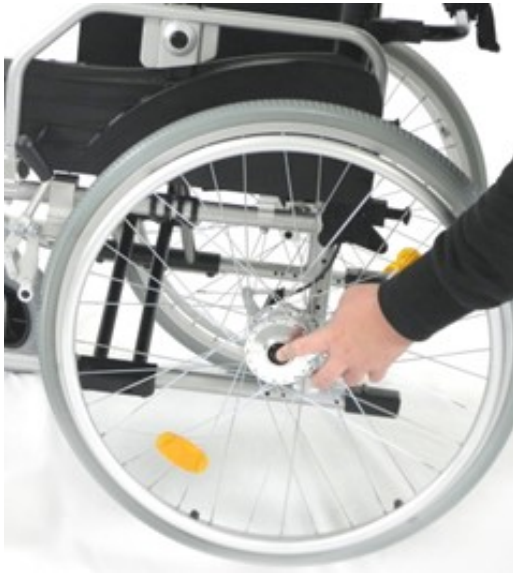
Fig. 7: Disassembling the rear wheel
