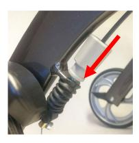
2. Re-tighten the Bowden cable by turning it anticlockwise or loosen it by turning it clockwise.
