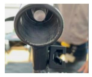
Screw on the nut. First tighten the screw lock and then tighten the nut with a **torque of 5 Nm**.
