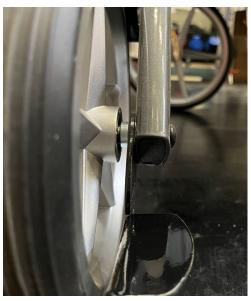
Tighten the nut of the rear wheel with a **torque of 5 Nm**.
